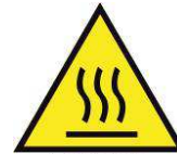
CAUTION HOT SURFACE
